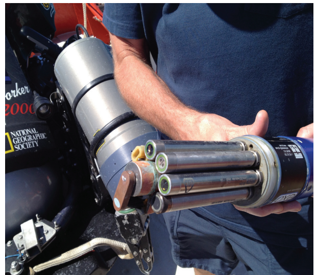
The new YSI EXO2 sonde features six user-replaceable smart sensors around a central wiper for easy calibration, maintenance and deployment.
