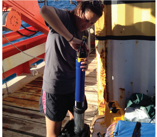
The new YSI EXO2 sonde is a completely new multiparameter water quality monitoring platform. Fully sealed construction and new engineering ensure even more efficient deployments, easier calibration and dramatic reductions in operations and maintenance costs.
