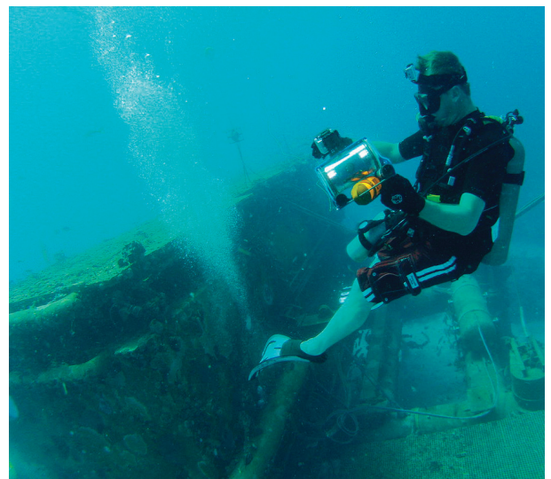
A rugged, bright-orange CastAway CTD continually gathers temperature, depth and salinity data as a diver explores a wreck.
