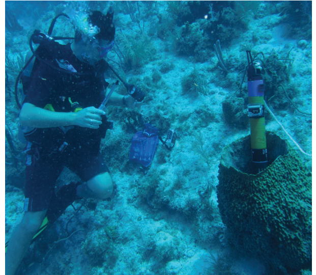
A YSI EXO2 multiparameter sonde provides an intimate look at water quality parameters inside a barrel sponge off the coast of Key West.
